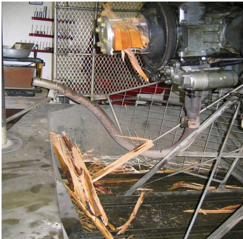
Right: Wooden propeller exploded when a wave came over the back transom from a misjudged levee crossing attempt.
