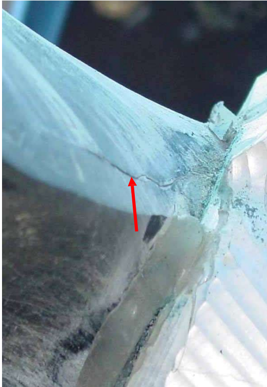
Above: Remains of a screwdriver that was forgotten on top of the motor after performing routine maintenance. Damage to propeller and oil cooler.
