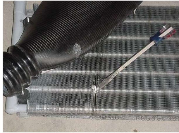
Above: Remains of a screwdriver that was forgotten on top of the motor after performing routine maintenance. Damage to propeller and oil cooler.
